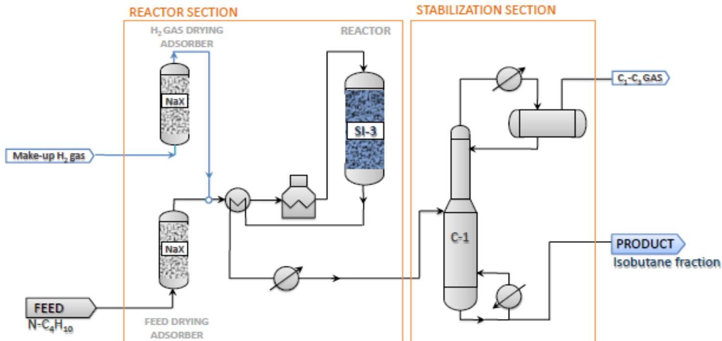
Typical Isomalk-3 n-butane isomerization unit consists of the following sections:
